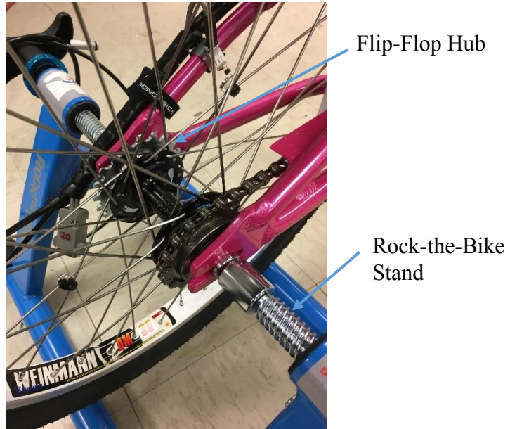
Figure 7: Rear wheel of large bicycle with flip-flop hub on far side of the wheel and the Rock-the-Bike attached to the axle of the bicycle.
