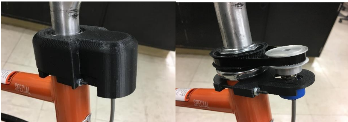
Figure 10: Potentiometer mount with and without the cover (left and right, respectively).
