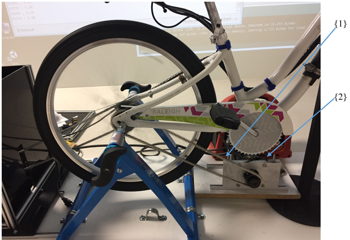
Figure 13: Experimental set-up for Experiment 1, Experiment 2, and Experiment 5. {1} Chain connecting the input motor sprocket and the rear wheel sprocket {2} input motor.
